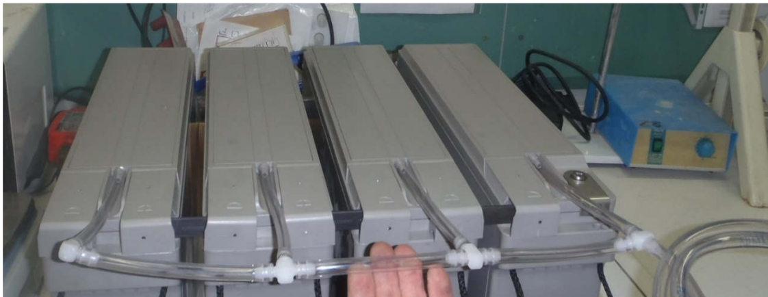
Figure 1– GAS evacuation system
